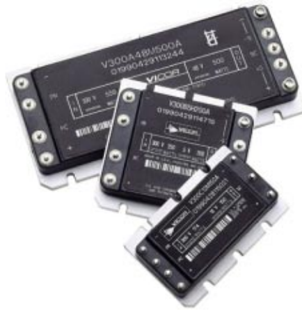
Figure 1. High-density DC-DC converters (bricks) come in full-, half-, and quarter-brick packages. The smallest module shown here measures 2.28 x 1.45 x 0.5 in (57,9 x 36,8 x 12,7 mm) and has a maximum output power of 150 Watts.
