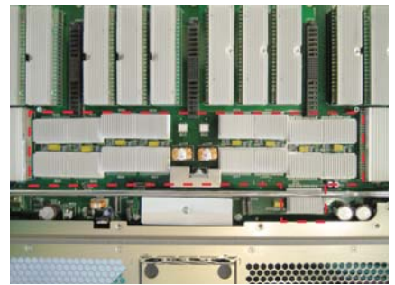
Fig. 5. An array of BCMs in IBM's p575 provides 5.1 kW at 11 V for the VRMs in the computer.
